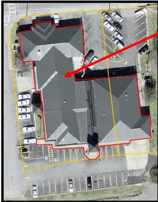
City engineers zoom in on the area so they will be working on the parcel close enough to identify the impervious surface.
